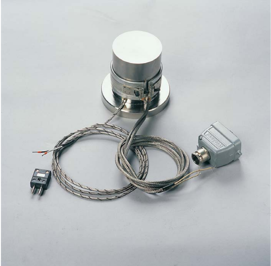
Figure 50. Band heater and thermocouple positioned on the upper punch.
