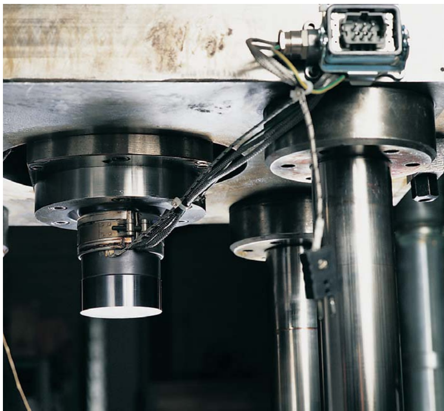
Figure 51. Upper punch fully mounted in tool set with heating accessories connected to a socket for quick-coupling.
