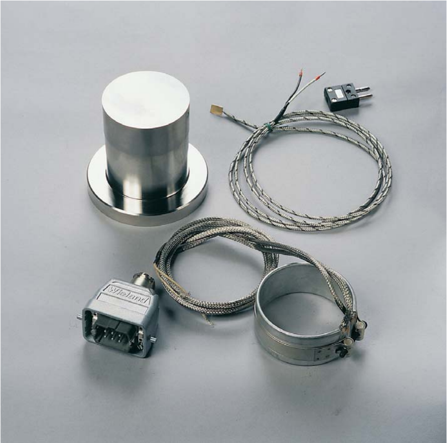
Figure 49. Upper punch and heating accessories (band heater, thermocouple and sockets).
