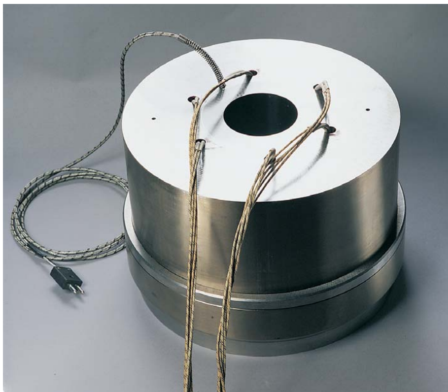
Figure 47. Cartridge heaters and thermocouple positioned in the die.
