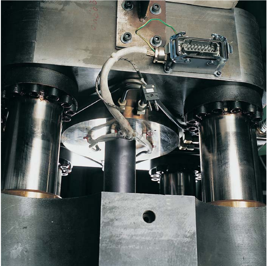
Figure 48. Die fully mounted in the tool set with heating accessories connected to a socket for quick-coupling.
